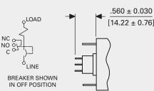
Auxiliary Switch (Note B) Two Pole
