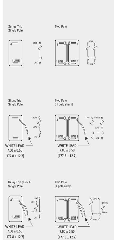
Note A: Coil Ratings to 5 amperes maximum. Contact ratings are 7.5 amperes at 50 Vdc and 250 Vac; 15 amperes at 120 Vac; 32 Vdc.
